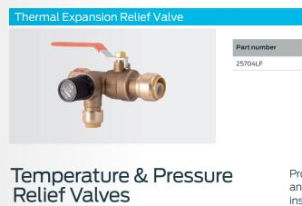
Provides temperature and pressure protection for residential water heaters and storage tanks. Push-to-connect design allows for quick and easy installation on copper and CPVC drain lines. Comes with standard factory settings of 150 psi for pressure and 210°F (99°C) for temperature relief. Completely automatic and reseats after temperature or pressure relief.
