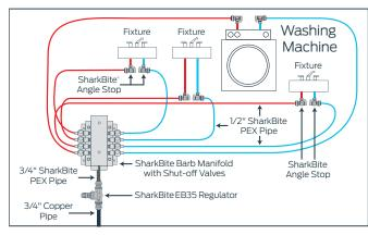
This system uses a central manifold to distribute water to fixture and appliances. One dedicated plumbing line is run to each fixture/appliance for both hot and cold supply lines.
