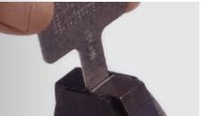
Step 1 Place GO portion of gage into jaw gap.
