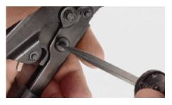
Step 3 Adjust clamp tool jaws by rotating the eccentric stud counterclockwise until jaws contact gauge. Re-tighten the locking nut.
