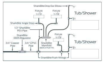
This system uses SharkBite push-fittings and manifolds offers additional versatility. When you need special-configuration fittings, such as drop ear elbows, SharkBite push-fittings offer greater speed and efficiency than traditional barbed fittings while costing about the same.
