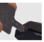
Gauge must stop at the NO-GO line in order to make proper
