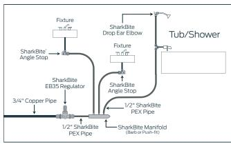
This system uses traditional PEX components (manifolds, barbed fittings, clamp rings, etc.) and offers the total lowest material cost. When you need special configuration fittings, such as drop ear elbows, SharkBite push-fittings offer greater speed and efficiency than traditional barbed fittings while costing about the same.
