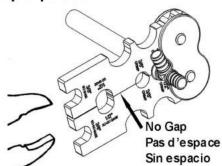
Squeeze the tool completely until the gap is eliminated in the area shown. When crimp is complete open the tool and remove the crimped fitting.
