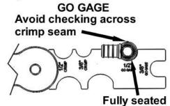
If the crimp ring is fully seated then check crimp in the NO-GO gage.Crimp should not enter and there should be a gap at the bottom of the nest.
