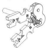
Open the tool (as shown above) and place it over the un-crimped ring. The tool must be centered over the ring. Take care not to reposition the ring during this procedure.
