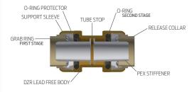
Only when the pipe has passed through the o-ring and reaches the tube stop is a secure joint created. The SharkBite fittings can only be used with pipe/tubing certified to the following specifications:
